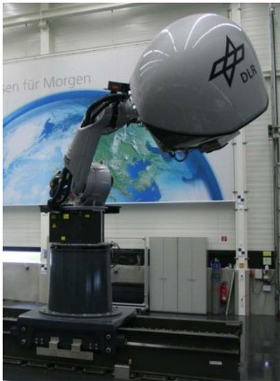
Figure 4: The DLR Robotic Motion Simulator
