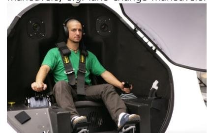
Figure 6: The simulator cell in flight simulator configuration (instrument panel removed)
